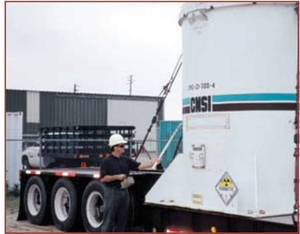
DHEC inspector performs radiological survey of transport vehicle upon receipt at the Barnwell facility.
